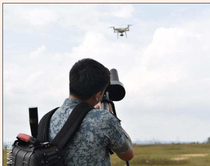
*A RSAF soldier holding a Jammer Gun, which uses signals to jam the control signals of a drone.*
