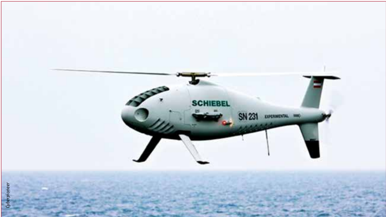
The Camcopter S-100, which sports state-of-the-art sensor systems, is used primarily for surveillance.
