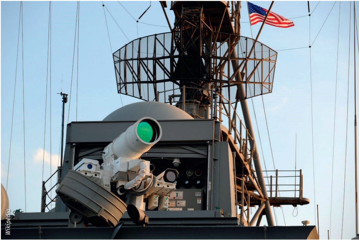
Figure 4: LaWS is the first operationally deployed HEL weapon and is installed aboard the USS Ponce.
