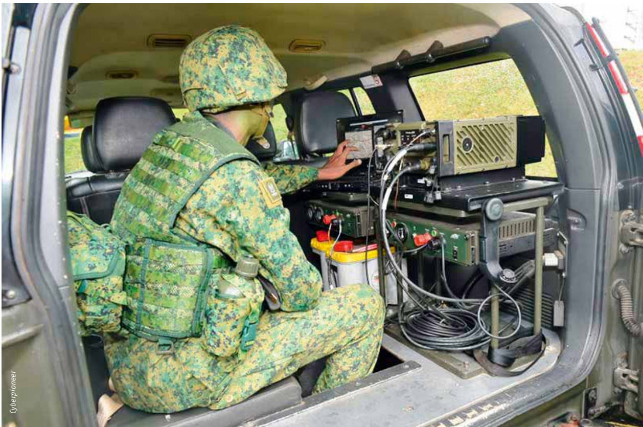
2WO Sathiaseelan operating the Software Defined Radio (SDR) mounted on an Operations Utility Vehicle.
