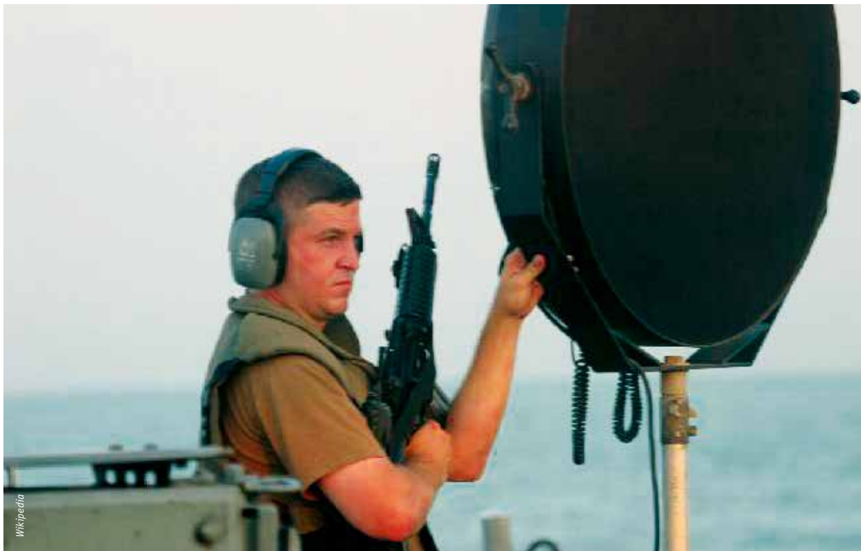
Long Range Acoustic Device capable of producing directed blasts of high volume sound waves.
