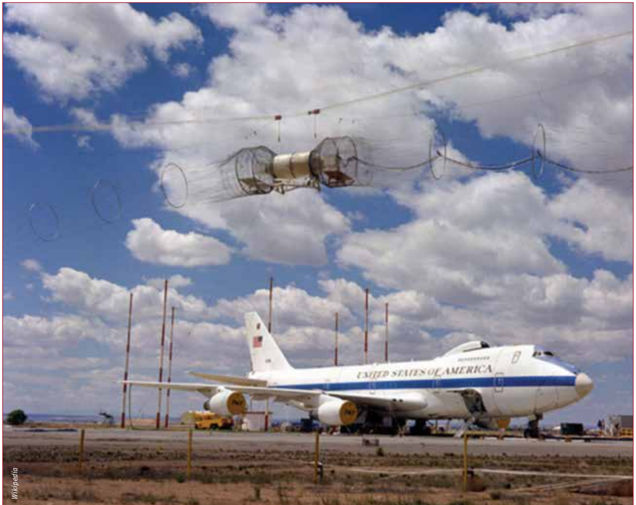
An EMP simulator HAGII-C, being tested on an American E-4 aircraft.
