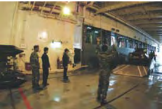
Well dock operations in the LST allowed fast landing craft to move in and out of the ship regardless of the tide.
