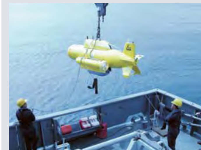
▲ "Yellow Submarines": Mine Disposal Vehicles, which look like miniature yellow submarines, are used to detect, locate, identify and destroy modern sea mines.
