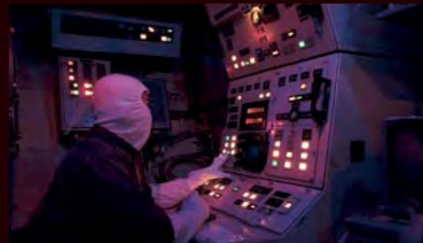
From Hands-On to Almost Hands-Free: The complex button-pressing sequences required to fire missiles on board the MGBs have been replaced by automated processes on board the frigates – the specialist only has to approve the engagement.
