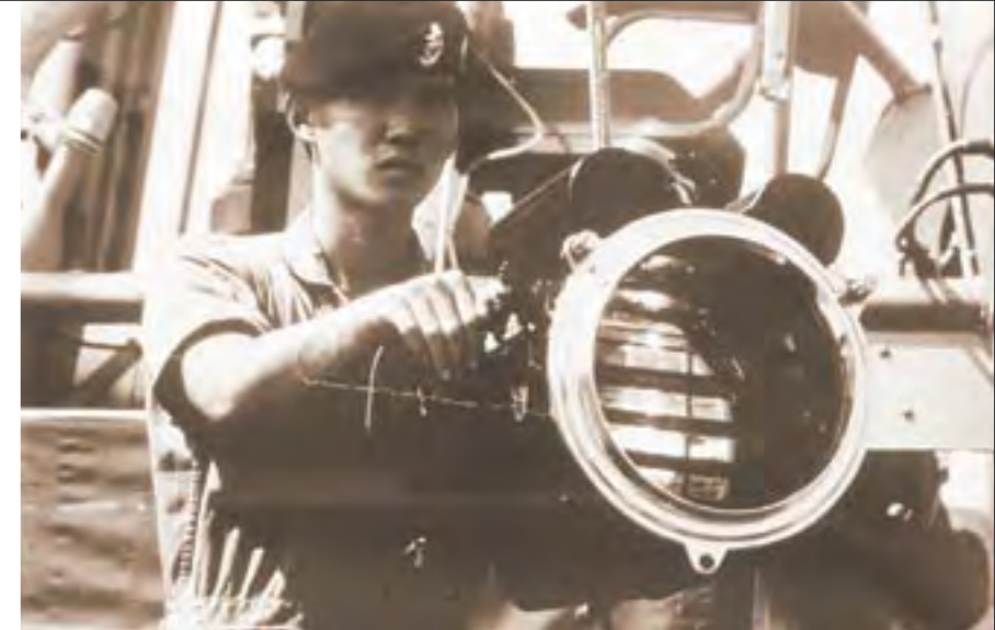
▲ Life Before SMS (Short Message Service): Communicating with other ships via visual signalling. But some things do not change. Flashing at sea remains a time honoured skill that continues to be practised by navies the world over.
