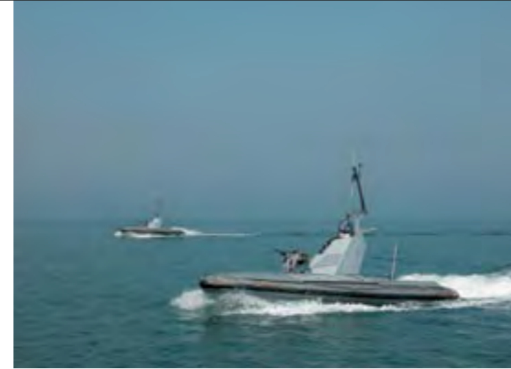
▲ Double the Protection: The two Protector Unmanned Surface Vessels (USVs) shown in this picture are capable of performing varied tasks such as identification and interdiction of threats at stand-off distances.
