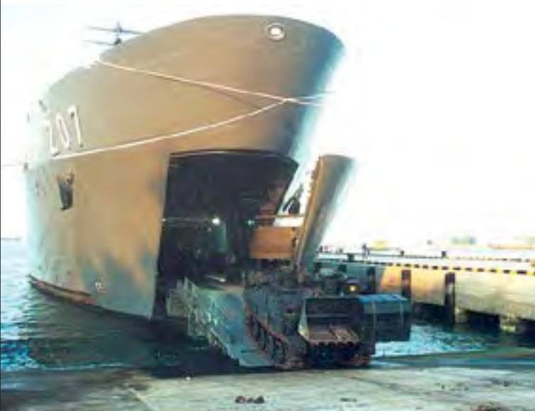
◀ Rolling On and Rolling Off: The Endurance -class LST can have vehicles and cargo driven onto her Tank Deck via a ramp at the bow of the ship.
