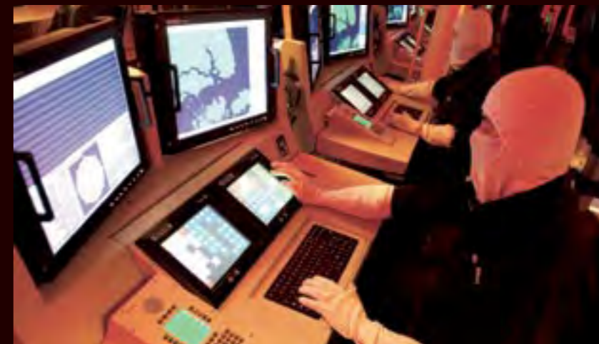
From Hands-On to Almost Hands-Free: The complex button-pressing sequences required to fire missiles on board the MGBs have been replaced by automated processes on board the frigates – the specialist only has to approve the engagement.
