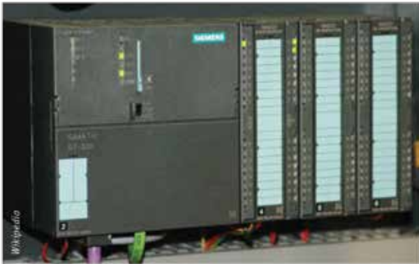
An example of the Siemens Simatic S7-300 PLC CPU that was infected by Stuxnet.
